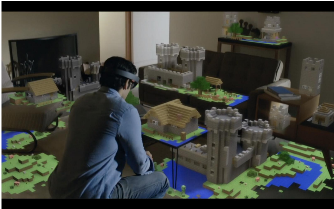
The virtual objects in the game can be placed correctly on the furniture in the room, because Hololens scanned the room's point cloud data in advance.
