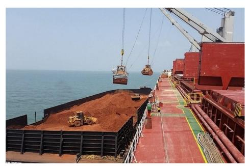
The bauxite that we will extract will be shipped to Aluminum refineries in China. The mining process is rather simple. We will give you a sneak peek into it in a later section. In the picture we can see crushed bauxite being onloaded to ships for delivery to China.
