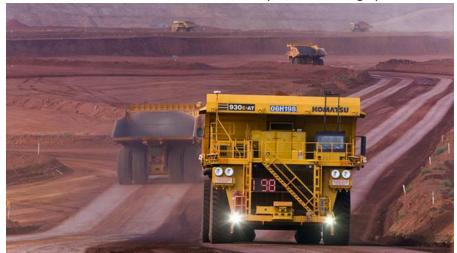
mining pits will be 3 m deep. The mining pits will be dug using bulldozers. The bauxite deposits will have to be ripped using drillers or bulldozers. Then they will be carried onto the crushing site using tippers. These will be prepared for shipment to refineries in China in the crushing site.
