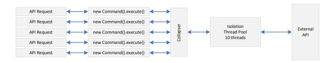
Request collapsing can be used to reduce the number of threads, and network connections needed to perform concurrent external API calls. Portus does this in an automated manner which does not require additional coding or manually batching requests.
