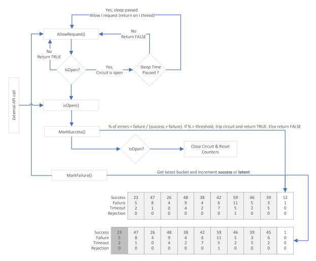
On GetLatestBucket() if the I-second window passed, a new bucket is created. The rest slide over and the oldest one is dropped.
